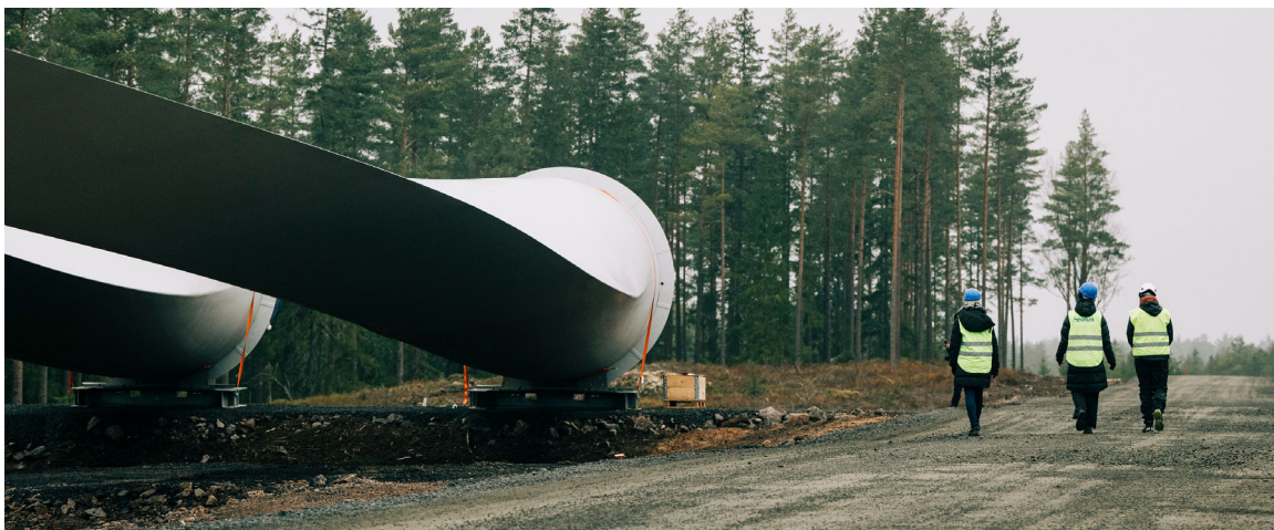
Turbine blades awaiting assembly at the Boarp wind farm in Vaggeryd municipality.
