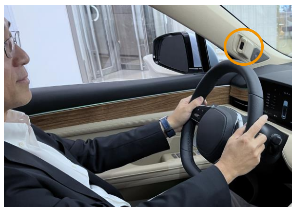
The photo shows an example of camera installed for facial detection.
