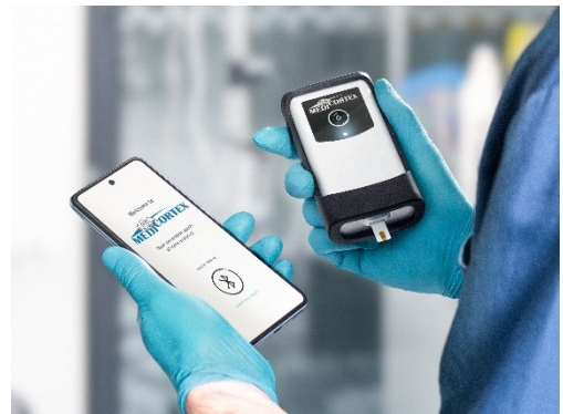
Figure 3. Illustration of the quantitative biomarker test based on an electrochemical sensor and a reader device.
