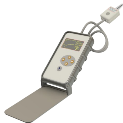
Figure 4. Outline design of a robust device applicable for repeated measurement of TBI biomarker level in saliva.
