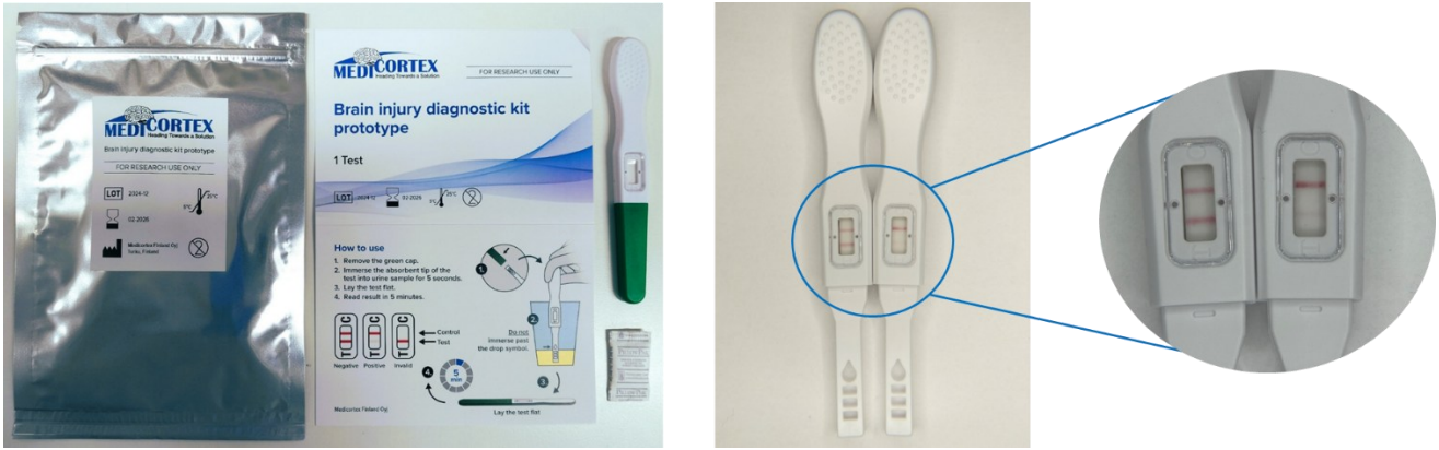
Figure 8. The prototype of the urine test kit incorporating a functional lectin-based detection strip was completed in the spring of 2025.
