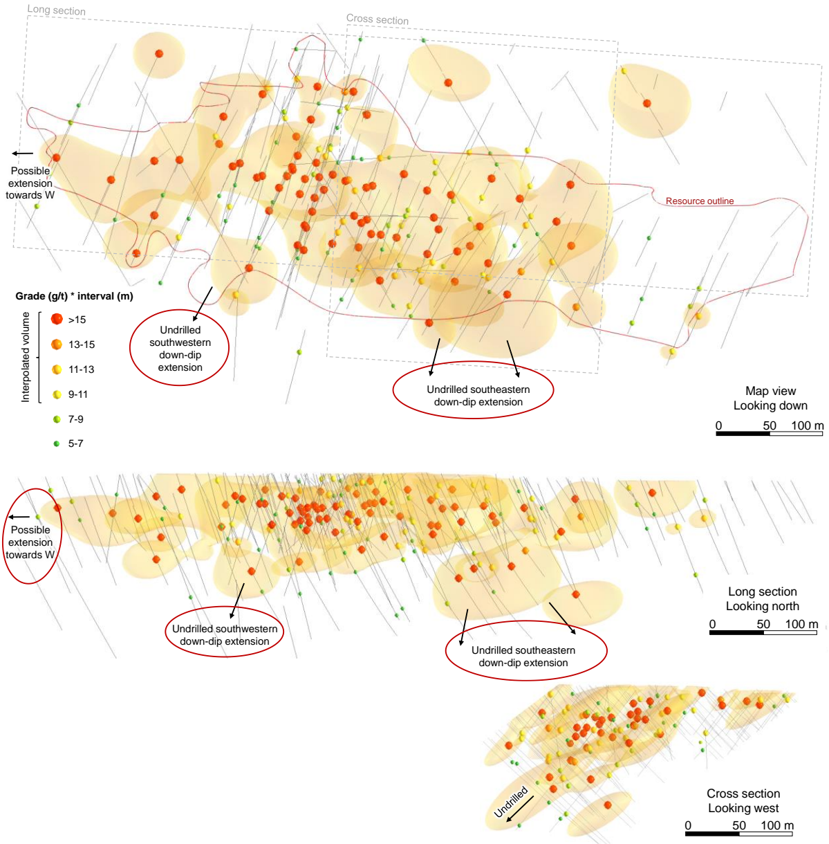
Figure 2: Kopsa gold metal factors (grade*intercept thickness) for drill intercepts exceeding 1.5 g/t Au, on map and long section (using LEAPFROG™ software), showing 2023 drill target areas
