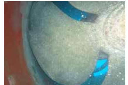
Coated vertical sides of the hull, uncoated bow thruster, uncoated azimuth propeller >26 months of idle time since ship delivery.
