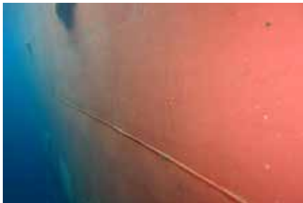
Coated vertical sides of the hull, uncoated bow thruster, uncoated azimuth propeller >26 months of idle time since ship delivery.
