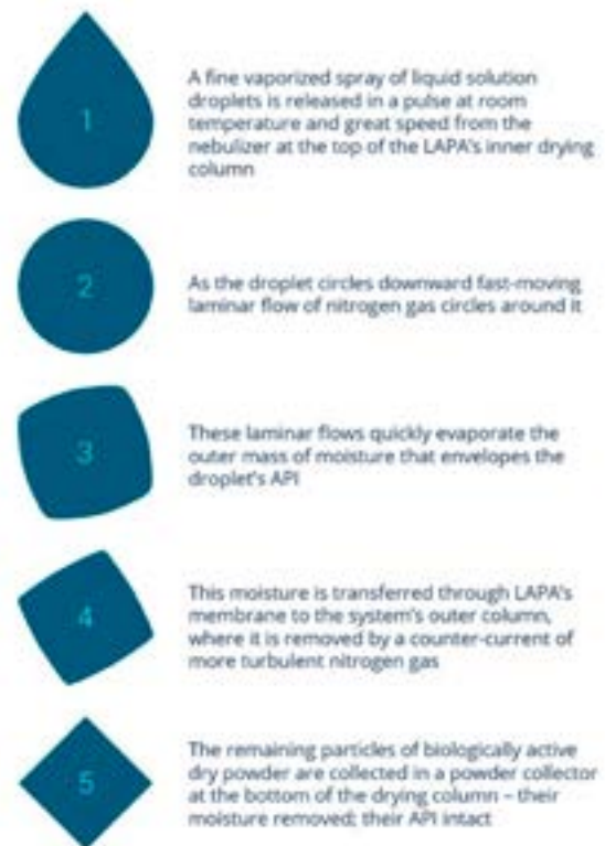
Illustration LaminarPace drying process of a single droplet of biomolecules in solution.
