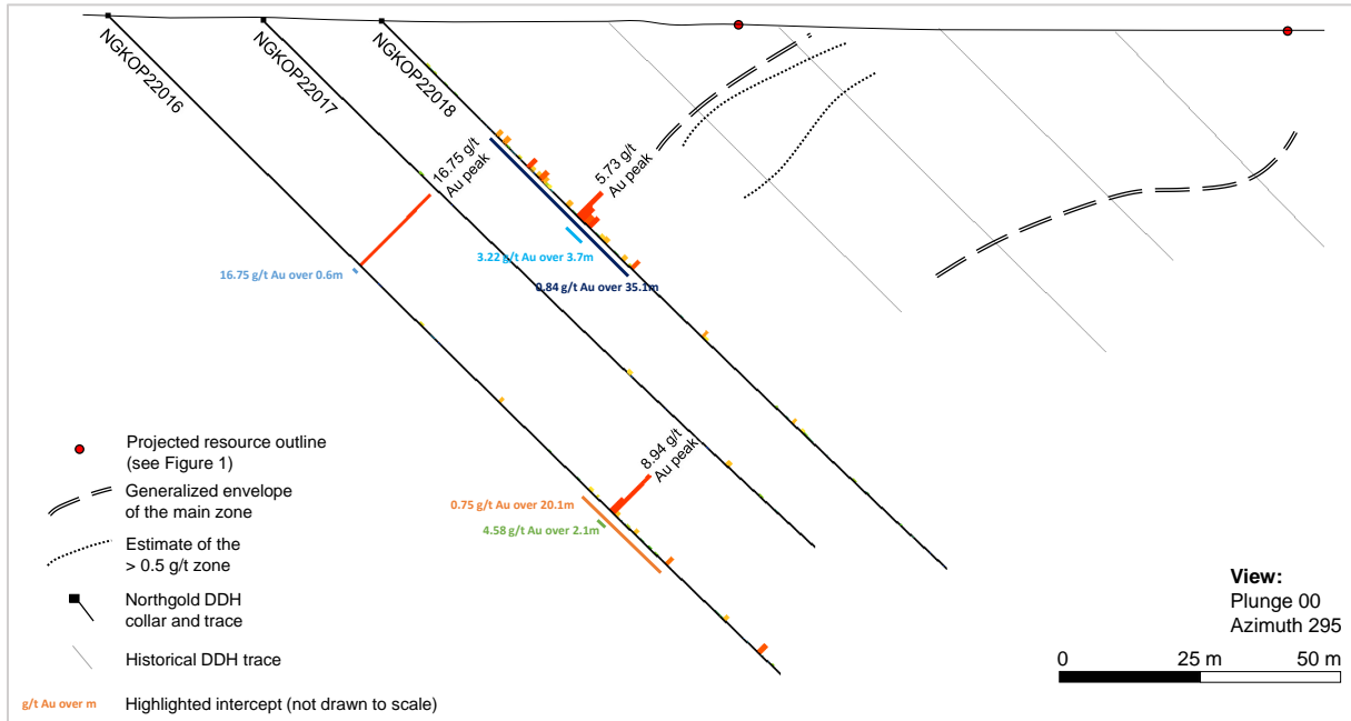
Figure 3: Cross section looking W-NW (using Leapfrog™ software) showing gold assay results for new drill holes NGKOP22016, NGKOP22017, and NGKOP22018 (60m wide slice)
