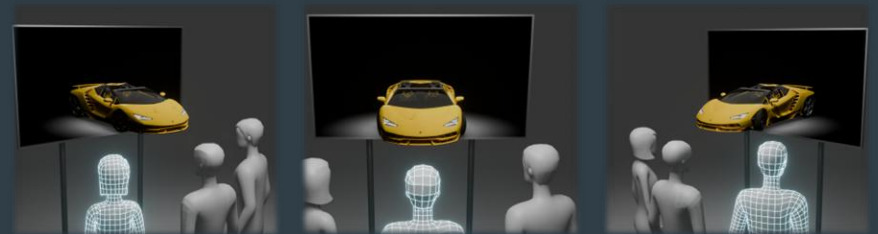
Example showcases the 3D multi-view function, allowing up to five users to see an individual view of the display
