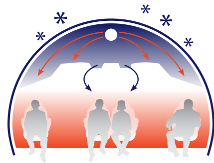
How it works: Humidity is added in the air duct to the cabin (blue arrows), providing a comfortable humidity level in the premium cabin. Dry air (red arrows) from the Anti-Condensation system prevents moisture problems.
