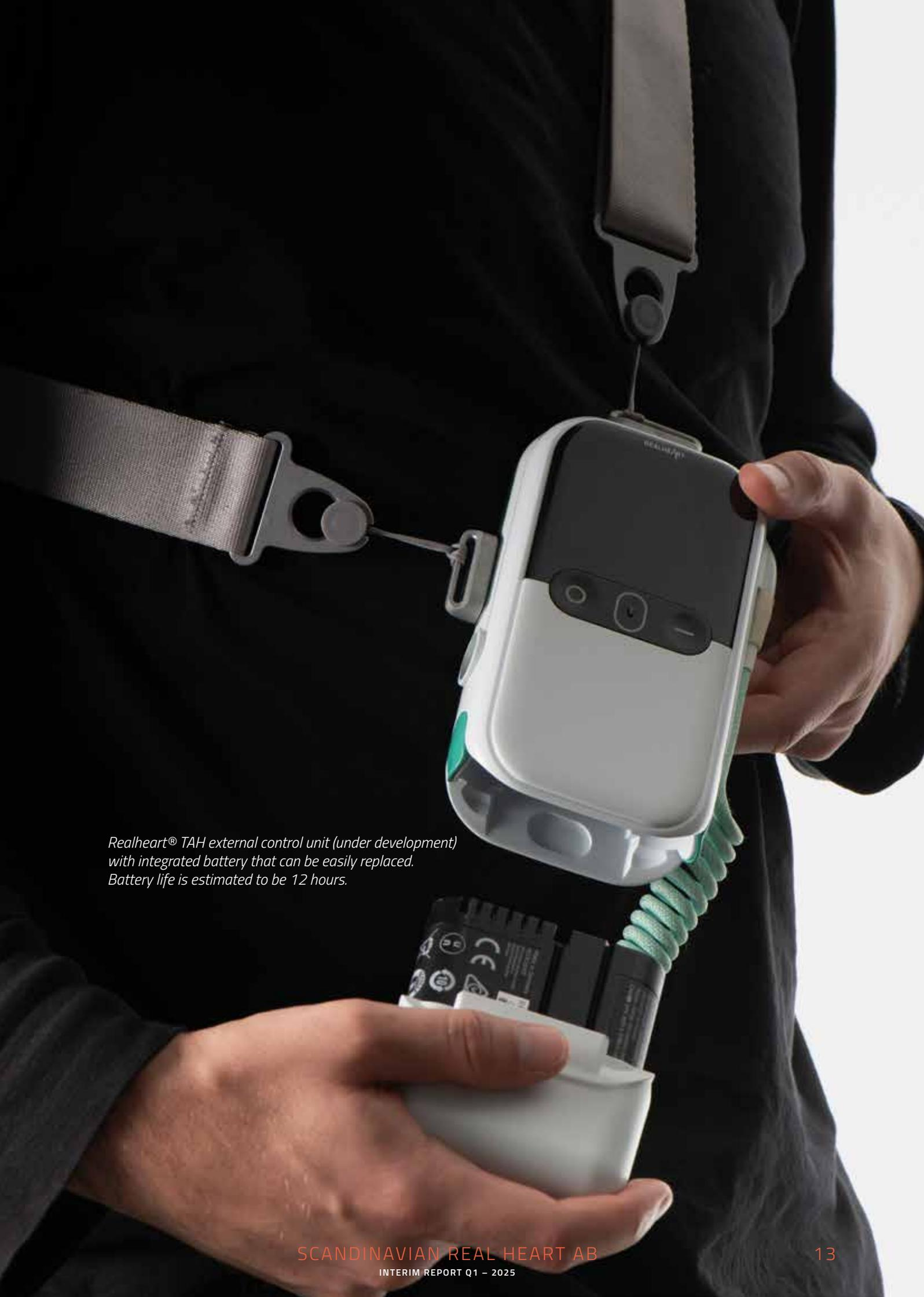
*Realheart® TAH external control unit (under development) with integrated battery that can be easily replaced. Battery life is estimated to be 12 hours.*
