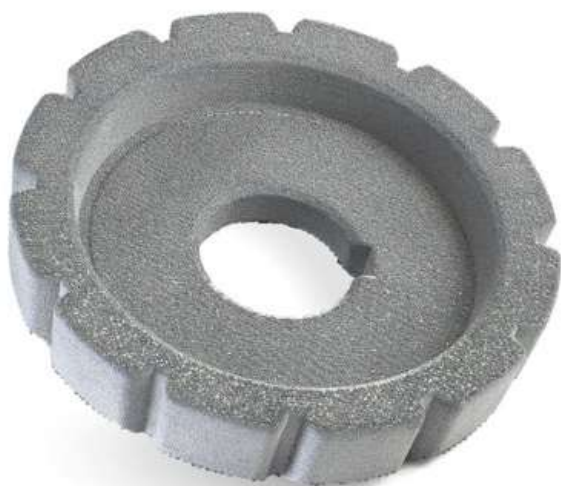
Fig. 7 A shape cutter (Ø 120 mm) in the as-built state, manufactured using PBF-EB by VBN Components AB from Vibenite® 290, an Fe/Co/W base material that combines high wear resistance and heat resistance. The component has a hardness of approximately 72 HRC (Courtesy VBN Components AB)
