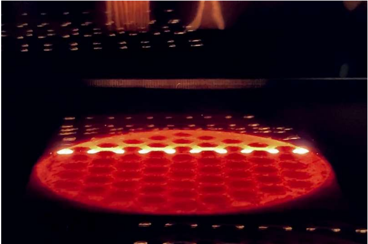
Fig. 3 PBF-EB processing enables a virtually instantaneous positioning of the electron beam over the entire build area of each layer (Courtesy Freemelt AB)
