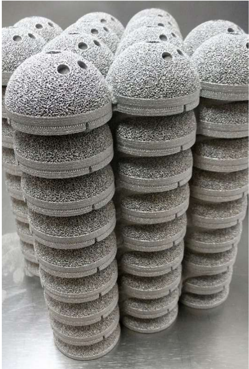
Fig. 5 Hip replacement cup implants tightly stacked with sintered powder between each part and no support structures (Courtesy GE Additive)
