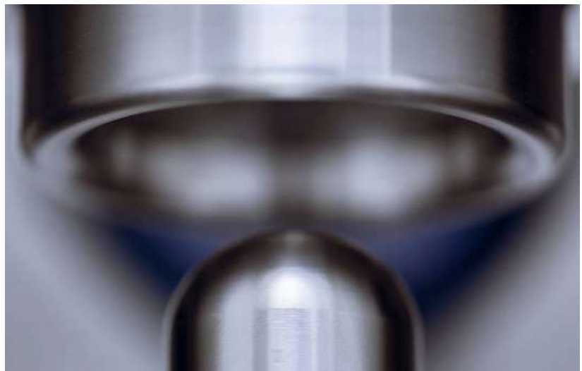
Fig. 4 Detail view of the electron gun on a Freemelt ONE machine (Courtesy Freemelt AB)
