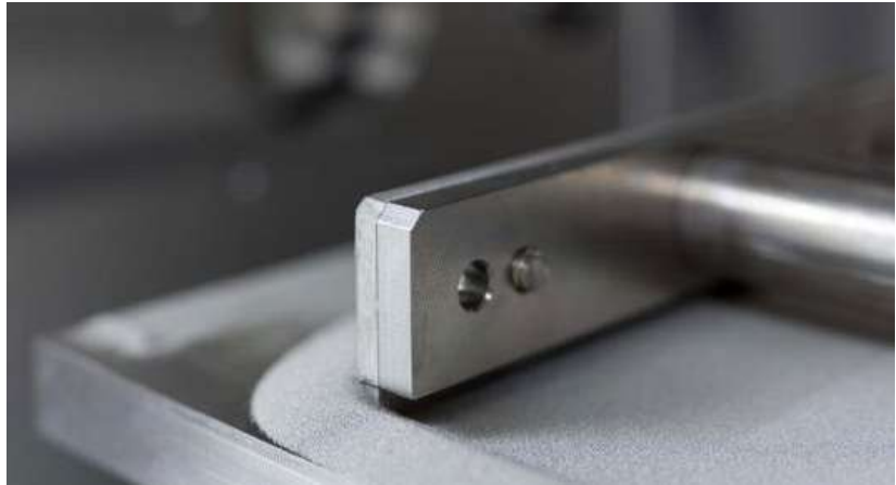
Fig. 3 The linear motion of Freemelt ONE's recoater is actuated by a mechanism positioned outside the vacuum chamber; this offers increased durability, since it is not exposed to extreme process conditions (Courtesy Freemelt AB)
