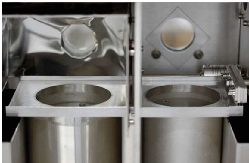
Fig. 1 View into the Freemelt ONE Electron Beam Powder Bed Fusion system's build chamber (Courtesy Freemelt AB)
