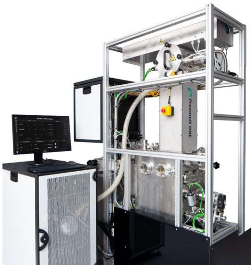
Fig. 2 Freemelt ONE's frame structure does not require an outer shell, giving open access to all ports on the vacuum chamber. If needed, this frame can be modified easily to connect third-party R&D equipment (Courtesy Freemelt AB)
