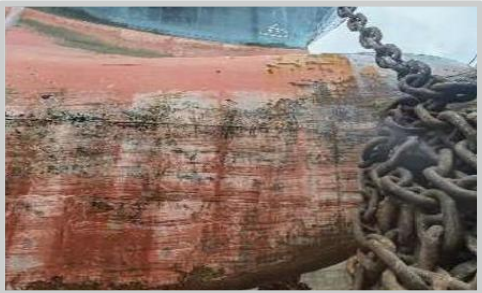
Image: "The report reveals that some of the hard animal fouling was on areas with coating breakdown"
