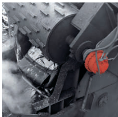
A car crusher needs a drive system that – in a tough environment – can be started and stopped quickly and can withstand shock loads.
