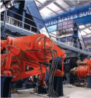
The crushing tandem at US Sugar's new line in Florida with the world's highest crushing capacity is driven by a system from Hägglunds Drives.
