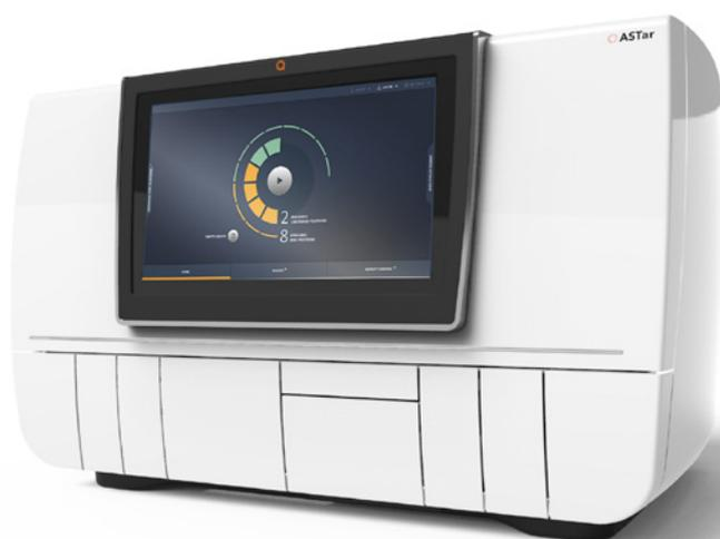
**The fully automated ASTar instrument** provides accurate and reproducible sample preparation for accurate MIC identification through a high-quality optical detection system. ASTar can be combined with a rapid identification system, thus meeting the clinical need for early and correct antibiotic treatment.
