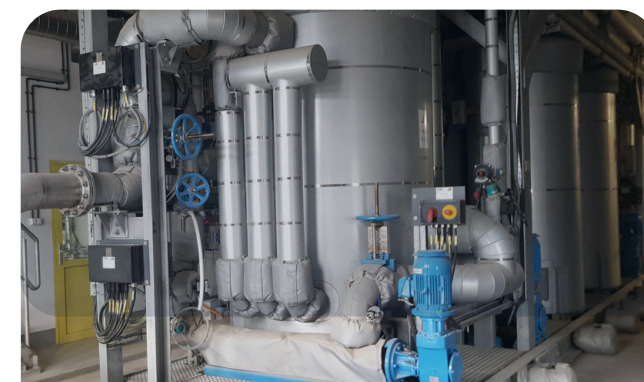
Cambi's first THP system in operation between two digestion steps in Warsaw, Poland
