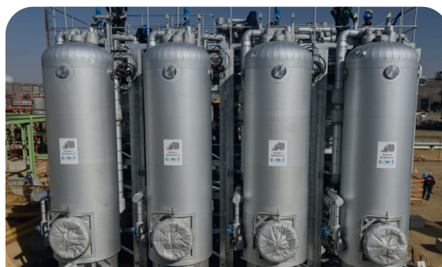
THP system for biological sludge installed at Sasol's industrial site in Secunda, South Africa
