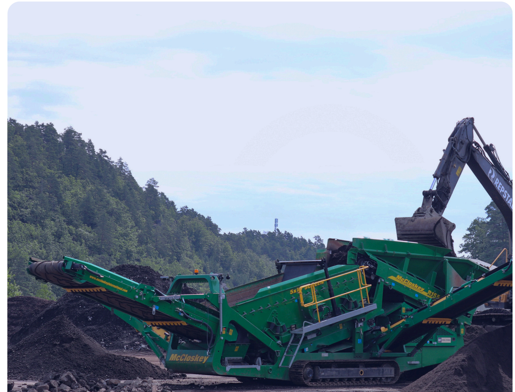
Bulk soil screener at Grønn Vekst's soil production site in Kristiansand, Norway
