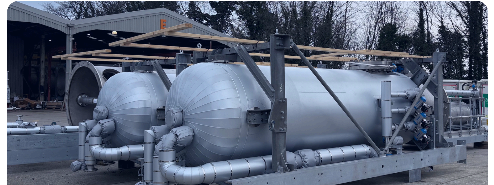
THP pressure vessels for the first model E system to be installed after anaerobic digestion for Veas near Oslo, Norway
