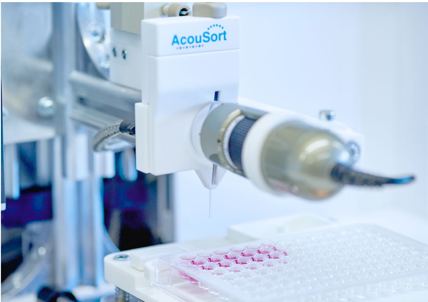
The AcouTrap chip, where cells or exosomes are trapped by the ultrasound, is mounted as the tip of a pipetting robot and offers live imaging of the trapping process.
