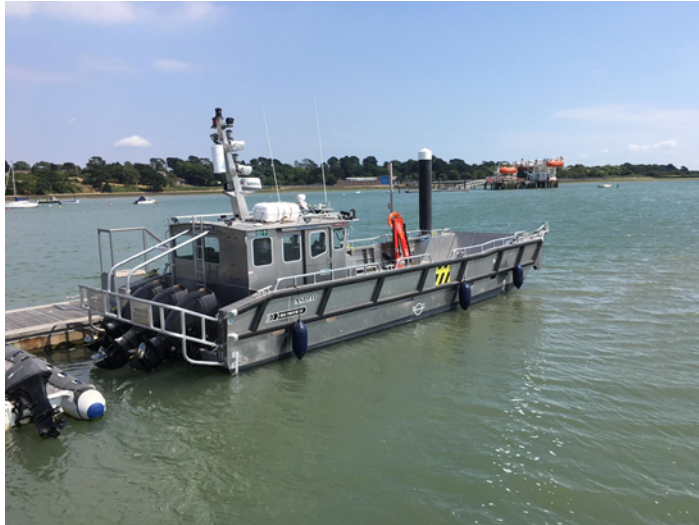
A recent triple installation of the OXE 150hp. The current work boat to be used on the River Thames where regulations only permit new boats to be powered by diesel engines
