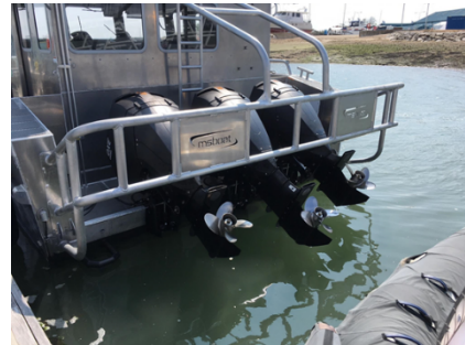
A recent triple installation of the OXE 150hp. The current work boat to be used on the River Thames where regulations only permit new boats to be powered by diesel engines
