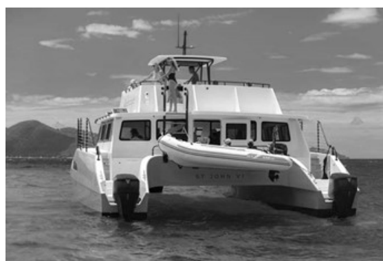
Above: The Voodoo Vi is a 57 feet long catamaran, powered by a double OXE200 installation. "The outboard diesel engines provide immense fuel savings over conventional gas engines. Generally, vessels this size have large inboard engines which require a lot of space, fire safety equipment, rudders and steering mechanics increasing draft and drag. Voodoo has no rudders and no machinery space at all as our power plants are outside the vessel making her very safe." - Voodoo Vi Catamaran Tours.
