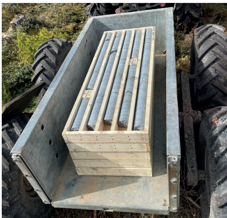
Fresh Kopsa core on route to the core shack for logging
