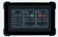
The new INVISIO Control app facilitates tactical communication management. It offers an intuitive interface with real-time visualization of all radio units connected to the intercom system. App users can see all traffic and user activity, manage access rights, change audio settings and relay radio communication.
