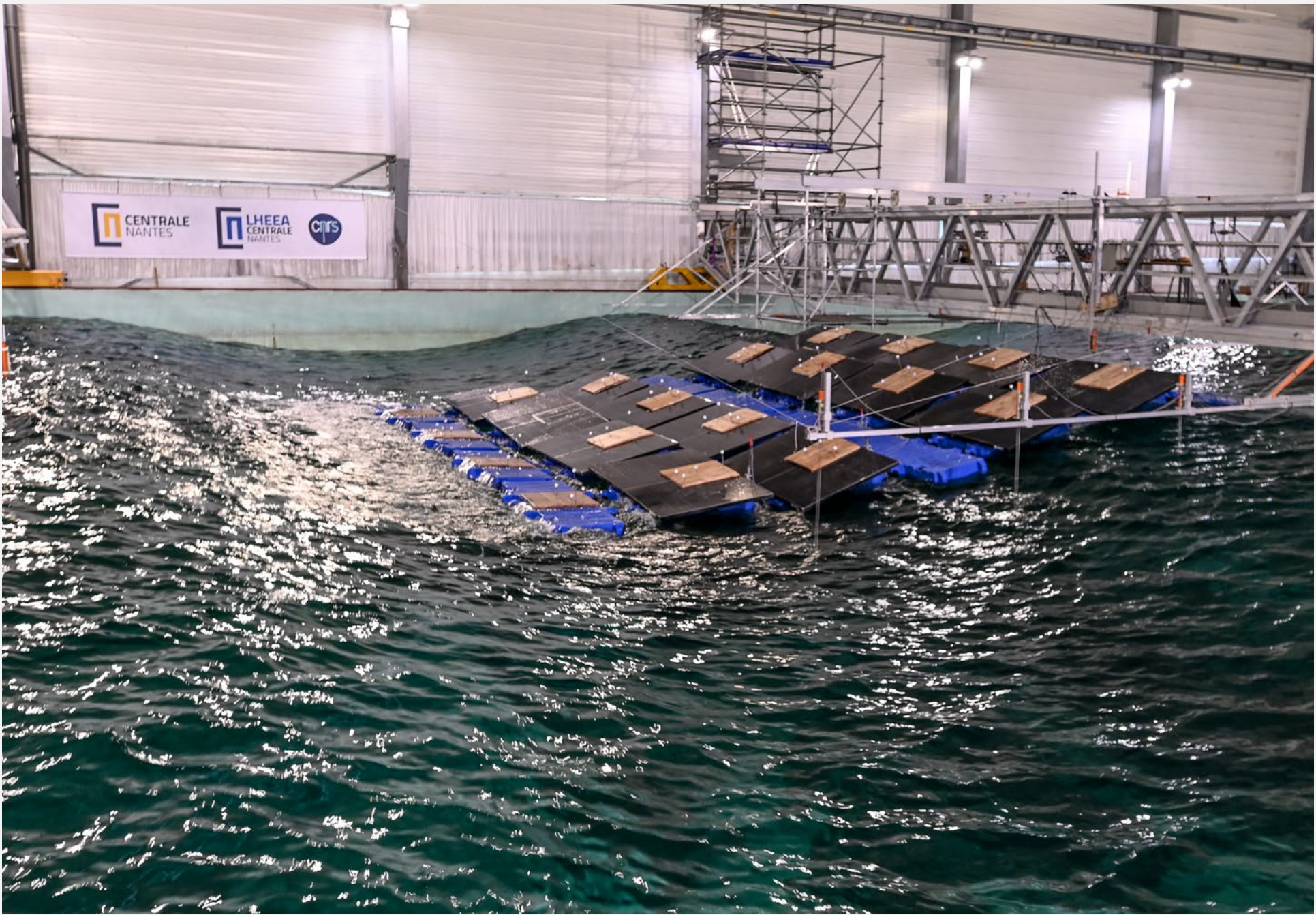
HelioRec’s latest design during the tests in the Centrale Nantes hydrodynamics and ocean engineering tank.
