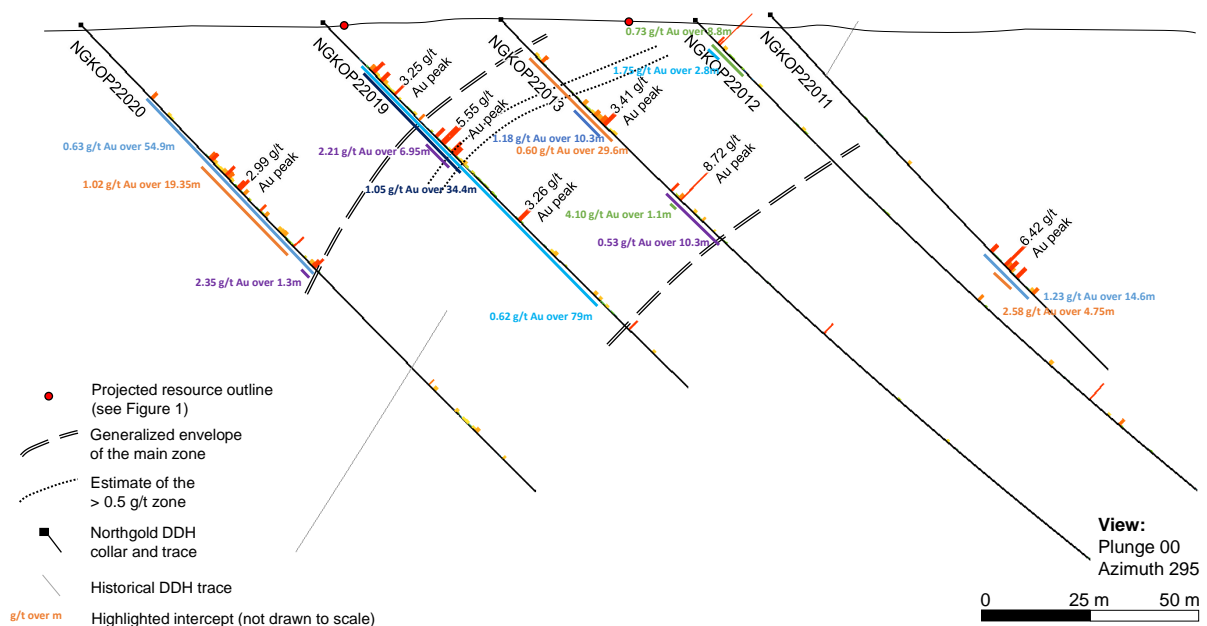
Figure 2: Cross section looking W-NW (using Leapfrog™ software) showing gold assay results for new drill holes NGKOP22011, NGKOP22012, NGKOP22013, NGKOP22019 and NGKOP22020 (50m wide slice)
