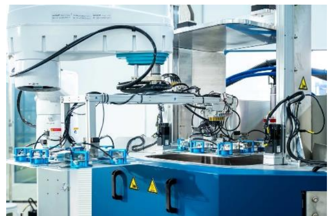
Coating of bipolar plates for automotive fuel cells at the company's coating center in Shanghai, China.
