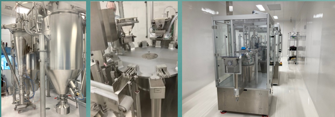
Images: Spray dryer and filling equipment used in Orexo's FDA-inspected production sites.
