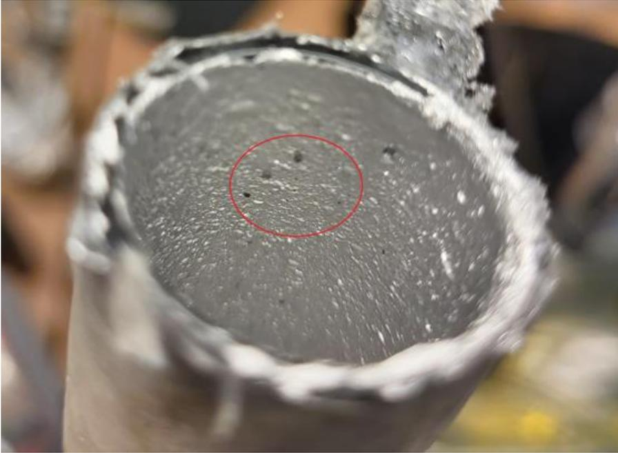
Image of solid carbon decomposed from carbon dioxide in the reactor tubes
