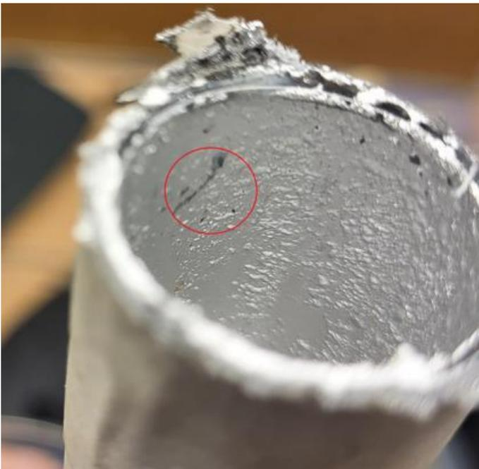
Image of solid carbon decomposed from carbon dioxide in the reactor tubes
