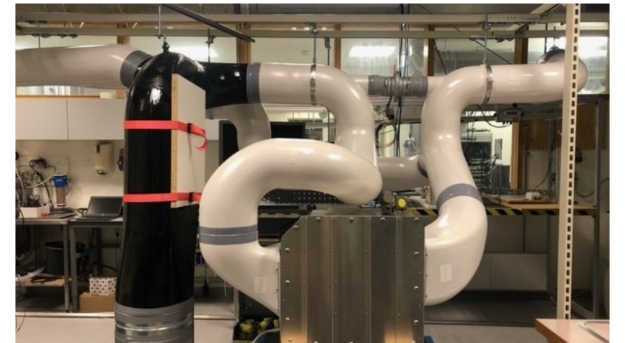
CFD (Computer Fluid Dynamics) analysis has been verified in CTT's system testing lab using a 1:1 scale model.
