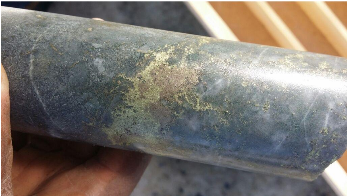
Plate 3: Example of MMZ showing intergrown bornite and chalcopyrite within highly altered core
