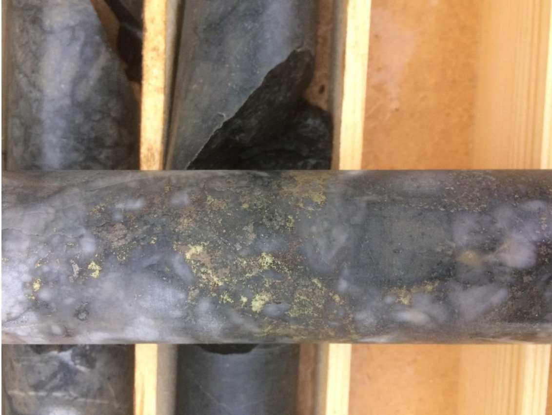
Plate 4: Example of MMZ showing intergrown bornite and chalcopyrite within highly altered core
