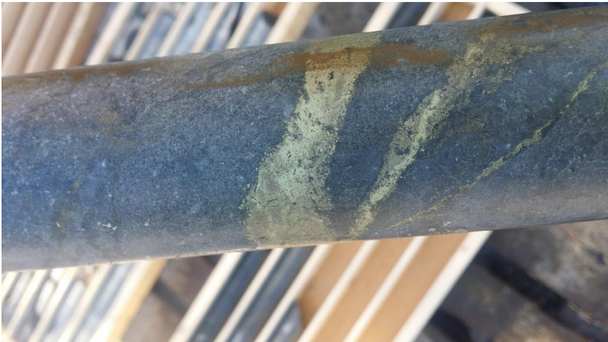
Plate 5: Example of MMZ showing veins of chalcopyrite pyrite and fine bornite
