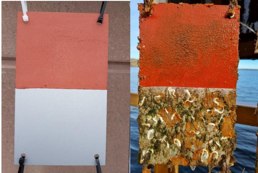
The picture on the left shows a panel whose upper half is painted with SeaQare™ paint. The lower half is unpainted and serves as a reference. This picture was taken at the start of the test. The picture to the right shows the same panel at the end of the test.
