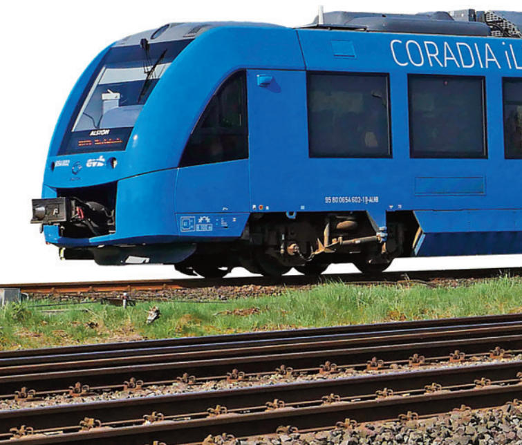
Coradia iLint, a regional train powered by hydrogen fuel cells.
