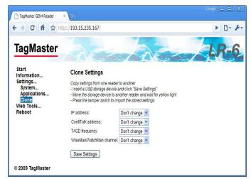
Reader configuration cloning using scripts downloaded to a USB stick
