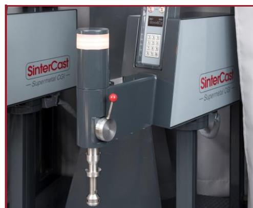
Re-engineered SAM with improved Thermocouple Holder
