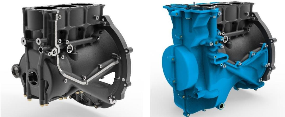
*Using high-strength CGI with durable composite outer casings, Tupy redesigned the cylinder block of a current-production 1.2 litre three-cylinder aluminium petrol engine to establish a cast iron solution with the same performance and the same weight.*
